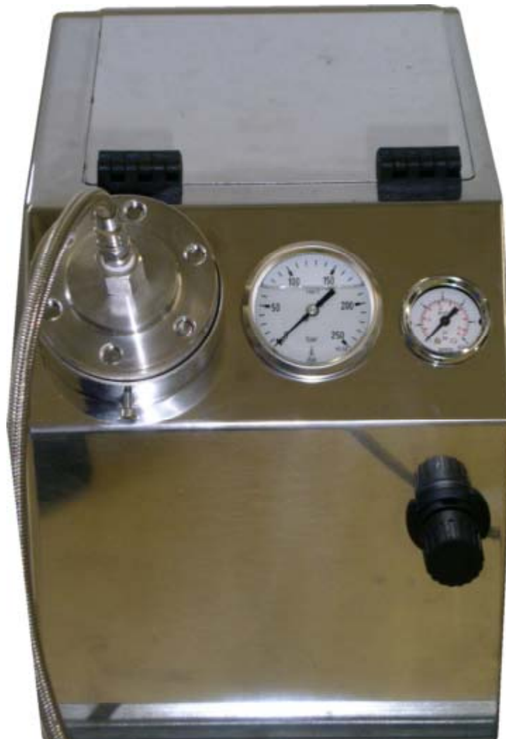
Figure 21: High Pressure Unit, outside
